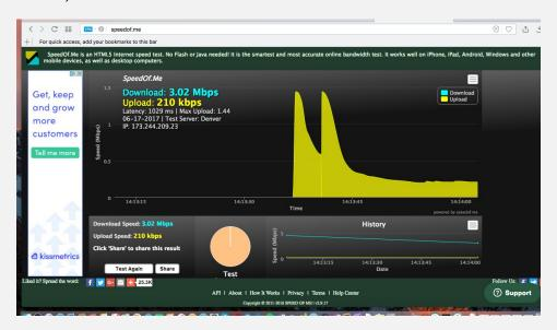
The latency here is about 10 times what is acceptable, which explains why pages are hanging when trying to load. The speeds are about half of what they should be as well.
